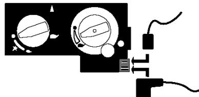
3. Connect the wires to the gas valve.
