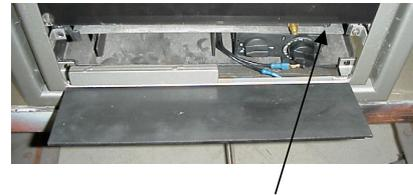
Fit a pressure gauge at the **test point** to check the setting pressure. The pressure should be checked with the appliance alight and at max. input. If the setting pressure is not correct then check the working pressure. After checking the pressure, turn off the appliance. Remove the pressure gauge and close the sealing screw. Re-light the appliance. Turn to max. input and test around the test point D for gas soundness using a suitable leak detection fluid.
