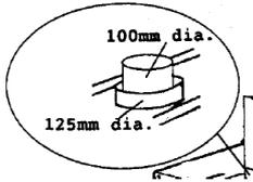
The flue connector outer collar is for connection to a 125 mm (5 inch) internal diameter pipe or liner. The inner collar is for connection to a 100 mm internal pipe or liner (see fig.)
