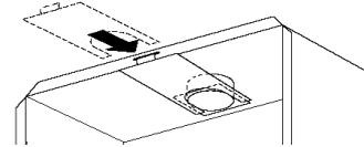
7. Slide the clamping plate with the lip upward under the vent connector. The flue connector and pipe or liner rests on the clamping plate. Make sure that the lip of the clamping plate goes in the slot on the front of the firebox (see fig.).
