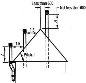
No part of the flue outlet shall be less than 1.5 m measured horizontally to the roof surface, or 600 mm above the ridge.
